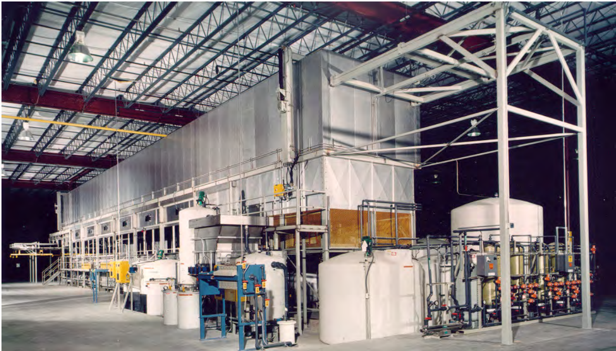
Figure 1. Square transfer indexing electrocoat system. Load/unload carousel conveyor is at the far end; cure oven is top, near end; forced cooling zone is top, far end. Water treatment equipment is in the foreground.
